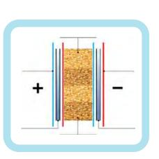
**Electrodeionization, EDI,** unites two proven technologies for producing ultrapure water: Electrodialysis and ion exchange. In contrast to conventional ion exchange in which resins must be either chemically regenerated or the cartridge discarded, EDI utilizes an electric current for continual resin regeneration.
