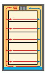
Our unique directed airflow design minimizes the risk of sample damage when the chamber is fully loaded
