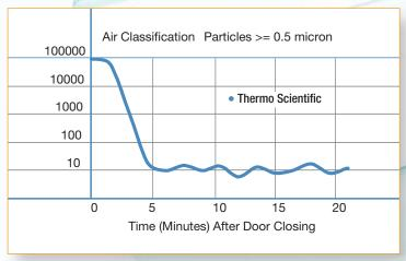
Security for your cells. The HEPA filter provides a 4 log reduction of particles in 5 minutes. ISO 5 clean room air quality achieved in 5 minutes from a door opening.
