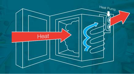
The TSX505's refrigerant loop absorbs and transfers heat energy from the outside into a heat pump in the back of the refrigerator. There, heat rejection coils transfer heat energy from the heat pump back into the ambient environment.
